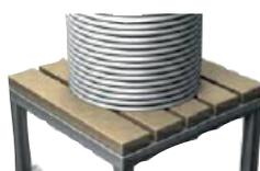
The top of the stand must be flat, smooth and level. Tank stands may be made with varying leg lengths to accommodate a sloping site. Kingspan Water tank stands are available to suit a range of tanks.
