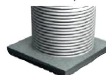
Slabs must be large enough to support all edges of the tank, and should be at least 100mm longer and wider than the tank. Slabs must be allowed to cure for at least five days prior to placing tank on slab.
